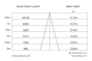
Due to the manufacturing processes of LED, the polar candela distribution and distance luminaries only reflect statistical figures and do not necessarily correspond to the actual parameters of individual product that may differ from the typical values.
