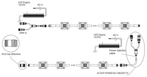
Power injection is required when the number of connected dots reaches the maximum value.
